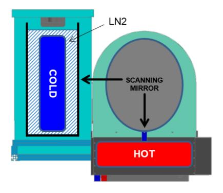
Fig.3.2: External cold load attached to the radiometer box.
