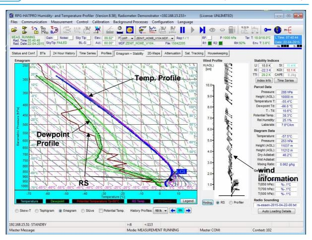
Fig.5.11f: Thermodynamic Diagram / Wind Info / Stability Index display.
