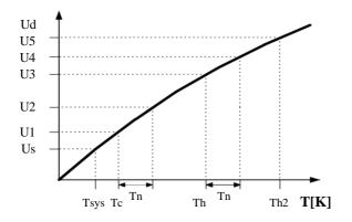
Fig.3.3: Detector response as a function of total noise temperature.  $T_{sys}$  is the system noise temperature,  $T_n$  the additionally injected noise,  $T_c$  the <u>total noise</u> when the radiometer is terminated with a cold load (e.g. liquid nitrogen cooled absorber) and  $T_h$  the corresponding noise temperatures for the ambient temperature load.
