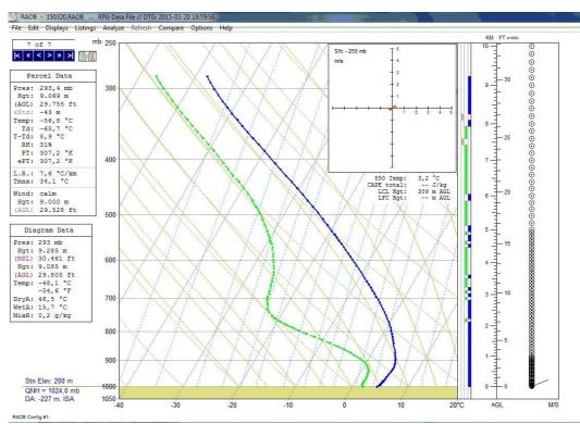
RPG-HATPRO profiles displayed by RAOB® (ERS), using automatically created RAOB data files.
