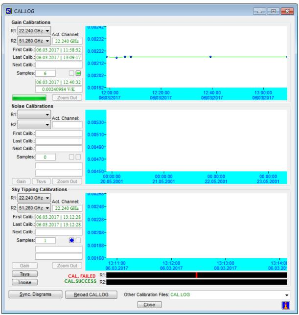
Fig.4.5a: Display of automatic calibration parameters.
